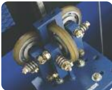
The low friction rollers eliminate the need for lubrication of the rails and at the same time enhance ride quality.
